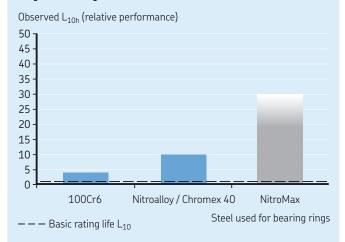
Note: Life test results depend on the lubrication conditions i.e. the values for the viscosity ratio  $\kappa$  and the film thickness to surface roughness ratio  $\lambda$ .
