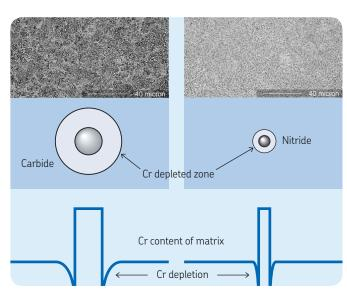
The microstructure of NitroMax steel (right) consists of a fine distribution of chromium nitrides, compared to the larger, brittle chromium carbides of conventional bearing steel (left).
